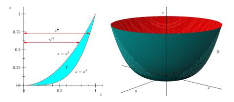
Figure 2.5.9: Region T rotated about z-axis to create solid body B
